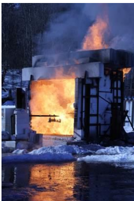
Photo of the large-to-full-scale jet fire test at SP Fire Research in Trondheim.
