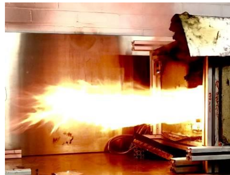
Bench scale backdraught experiments as part of the "Strategies for fighting fires in basements" project - a 1m long flame extends from a 1m long enclosure.
