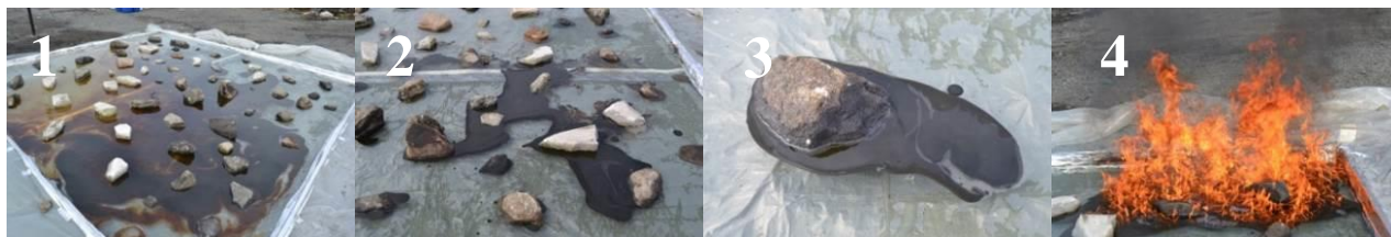
Experimental steps of in-situ burning of crude oil on water covered with objects. Spreading of oil (1), herding of oil (2), object interaction during herding (3) and burning of the main slick (4).
